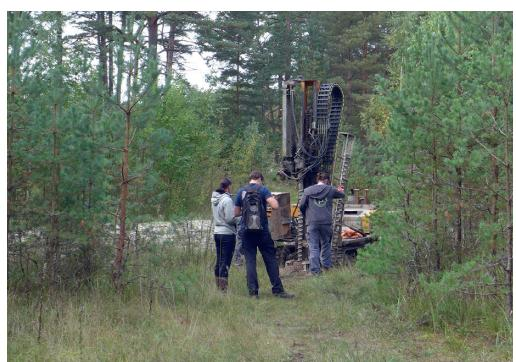
**Fig. 3.** Boring by machine for sampling in Pärnu.
