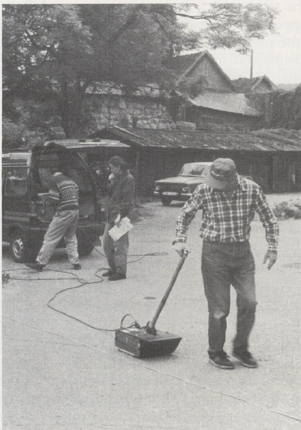
Fig. 2 The application of the GPR in the old town of Viljandi.
